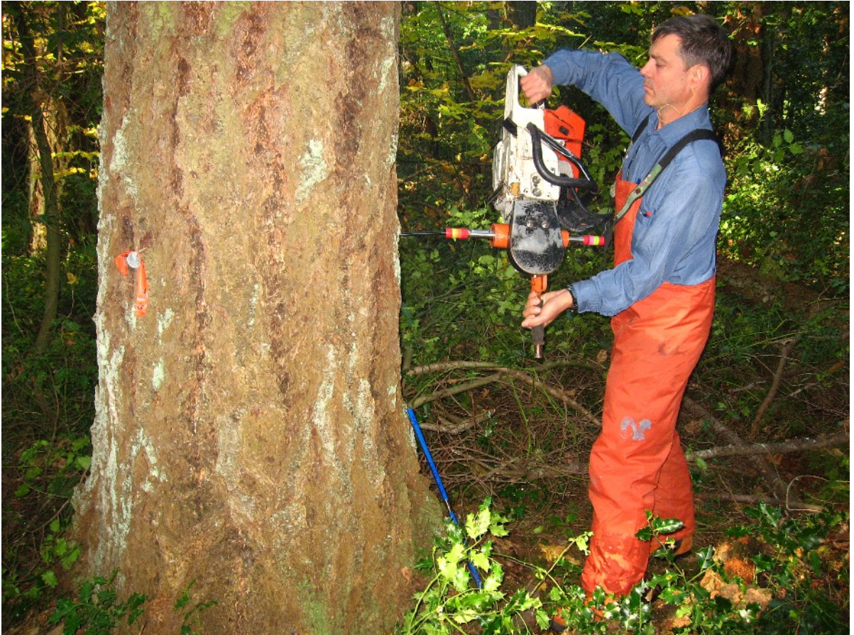
Ministry of Forests researcher Kevin Hardy takes a core sample using a custom drill he developed.
