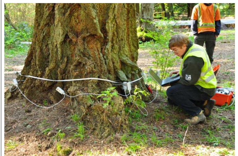
Transducers spaced around the tree send sound wave propagation data to a data acquisition system.
