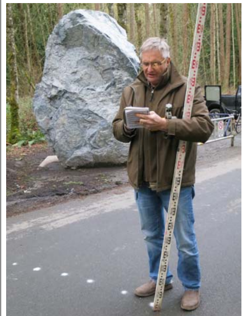
Illarion Gallant measures road slope for new leaf gate.
